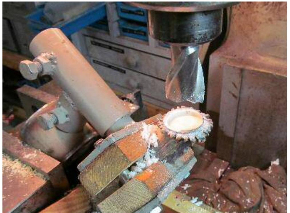
The result is depression with squared sides and a 1.125" depth just crying out for the cast piece.
