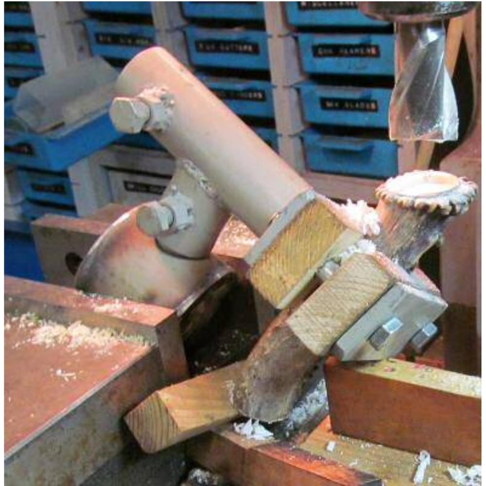
Add some epoxy to the seat, plop the casting in place and wipe off excess epoxy and you get a nice “pop”.
