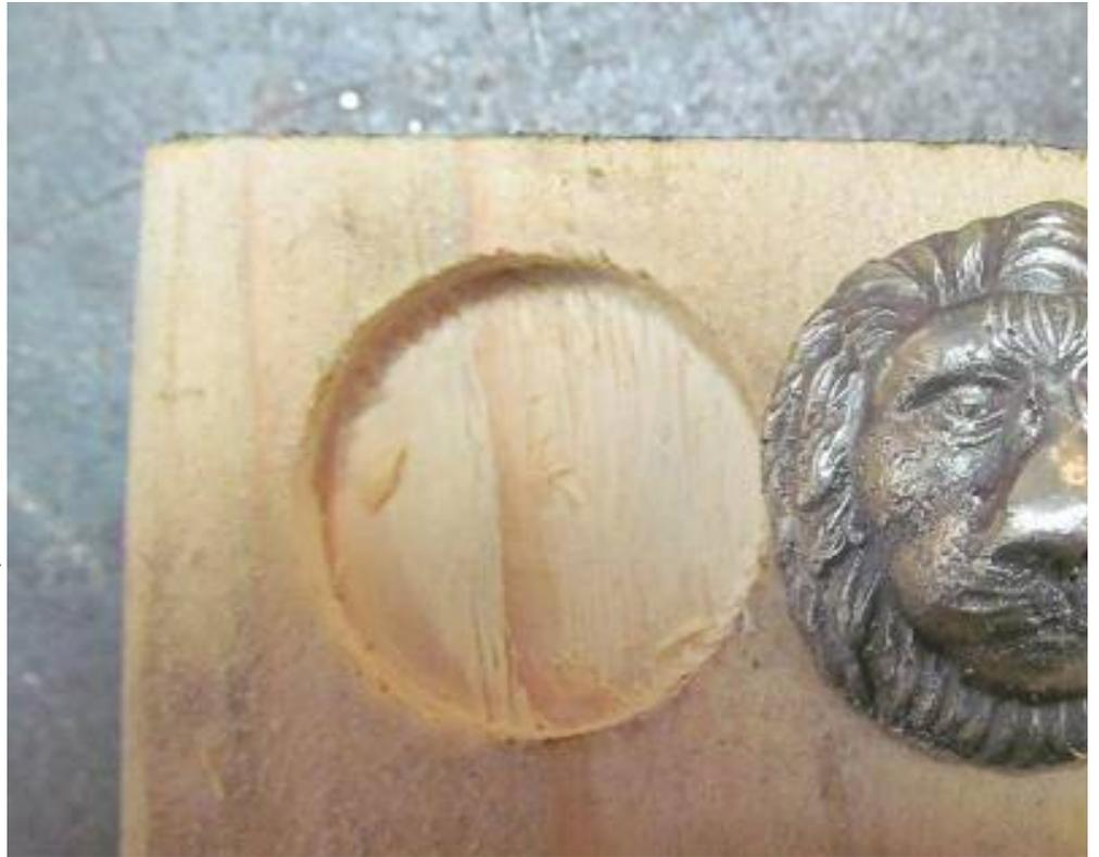
I used a plastic template for the scribe and then carefully ground away the edges of the casting until it just fits the trial depression. Voila.
