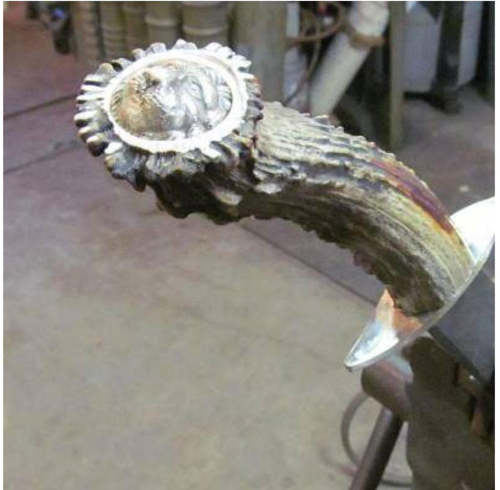
From my website, here is the documented appearance of the piece (the blade is 01-L6-1095-203E at 132 layers). It was austempered. The guard is nickel silver and...
