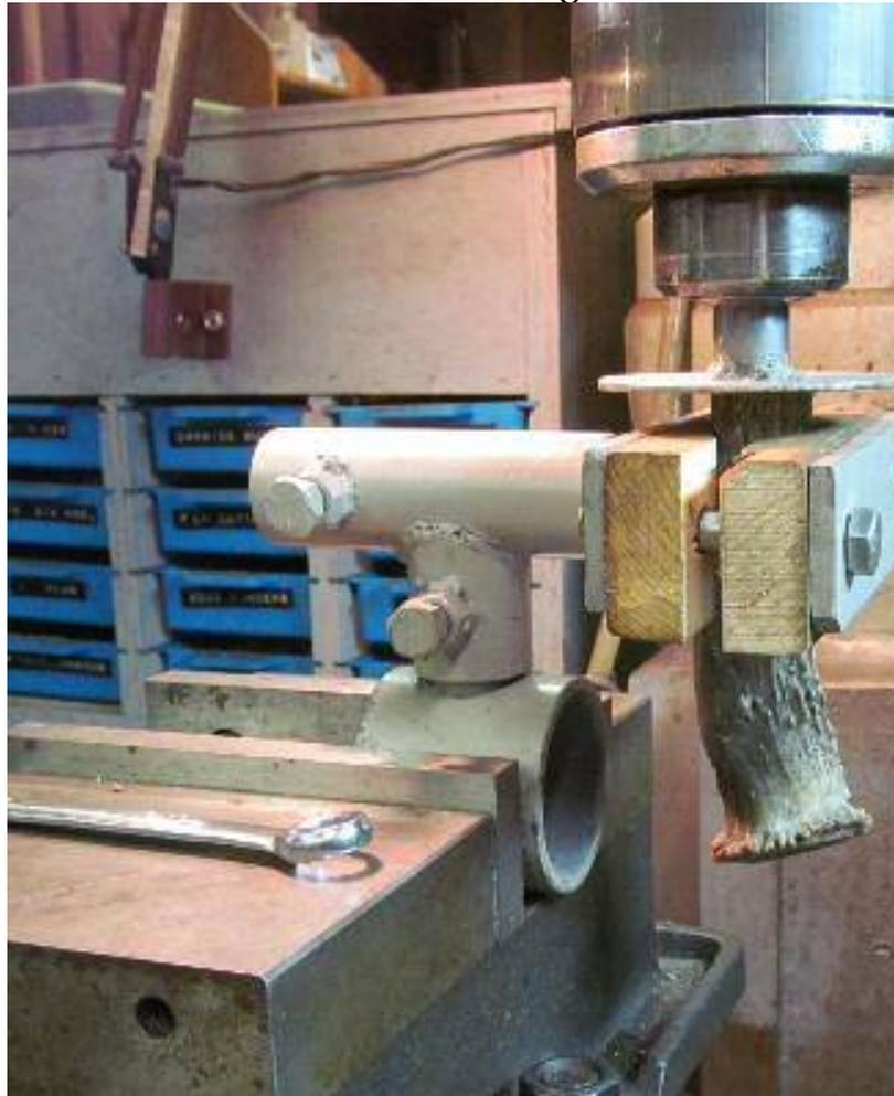
The third section has a set of wood “V” blocks to clamp – without damage- the stag. As long as the guard’s rear surface is parallel to the mill’s cutting plane, all is well.
