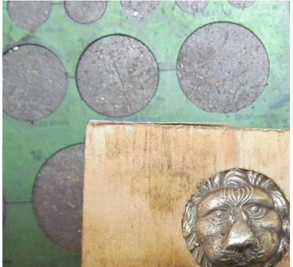
The jig was reset to place the crown's surface parallel to the mill's cutting edges (and some wedges were used to be really sure that nothing moved) and the real depression was made. Not clamping enough tends to be depressing....
